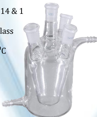
Gas-tight thermal jacket cell [KEC04V100]
